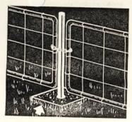
Our swinging gate sagged on one end when we used it across a wide opening so we decided to use two shorter gates and join them at a post in the center. A cement footing with a large diameter pipe in the center is poured at ground level. The smaller pipe, which serves as the gate support, is set in the larger pipe and can then be removed to let vehicles through the gate.—D. E. Illinois.
