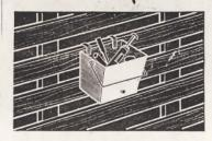
We made a handy holder for veterinary supplies by welding strap irons to an old nipple bucket. The bucket can be hung on the fence near where you're working livestock.—M. A., Kansas.
