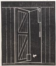
We use this weighted chain to close our farrowing house door behind hogs as they go in and out. The bottom of the door is reinforced where the hogs push it open.—G.S., Iowa
