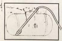
Safely fill spray tanks with a garden hose by using a 6-ft. section of 1½-in. galvanized pipe. The pipe reduces foaming and prevents hose damage from chemicals. A short piece of 2x2 bolted on the end prevents pipe from damaging tank.—
