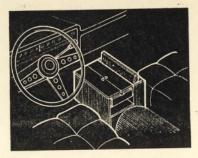
This center console keeps things from building up on the dash of my pickup truck. We built it with a slide-out drawer for small pieces, a slot to hold magazines and a lower shelf for larger items.—K. M., Illinois.
