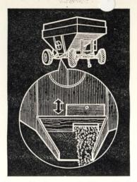
To easily dump grain into a 5-gal. bucket for filling planter boxes from our gravity-bed wagon, we cut a 2x6 to fit snugly into the dump tray. We cut a section out of one corner of the board to let the grain flow out. Any small, thin sheet of metal will work as a gate to shut off the grain flow.—J. B., Illinois.
