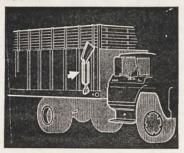
Keep shovels handy by welding or bolting a section of 6-in. pipe to the outside of the truck or wagon box.—
