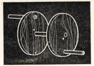
We wind wire easily with this spool made of ¼-in. plywood and steel pipe. A small hole drilled in each side near the center helps start the wire.—L. G., Pennsylvania.
