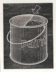
Prevent paint build-up on the top lip of paint cans by using an old lid, cut in half, to wipe excess paint off of brush while painting.—J. S., Illinois.
