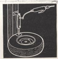
We made this tire bead breaker by mounting an old hydraulic cylinder to wall post in shop. We replaced oil ports with air valve stems with the cores removed and operate the cylinder with our air compressor. A curved steel plate is welded on the ram to apply pressure to tire.—J. K., Ohio.
