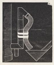
We fill our auger hopper from the vertical unloading spout on the grain bin with the aid of a 6-in. plastic drain tile. The tile is secured to the vertical auger with rubber straps. A 6-in. section of metal tube keeps the tile from collapsing at this point. The tile is easily slipped off the spout for loading trucks or wagons.—F.M., Minnesota.
