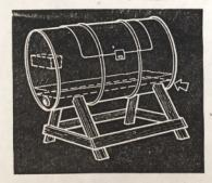
We made this parts washing tank by cutting a 19x24-in. section from the side of a 30-gal. drum. Then, we cut a 21x26-in. piece from another drum to serve as a hinged lid. Hardware cloth with ¼-in. holes keeps parts up off the bottom of the drum and a pan bolted to the side holds parts while they drain. —D. D., Illinois.
