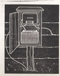
We built this portable fencer by enclosing a lead-acid battery and fencer unit in a plywood case. It can be moved to a new post in minutes by disconnecting the two wires.—J. H., New York.
