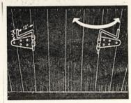
We store the stock racks from our pickup on these hangers made from old door hinges and %-in. steel rod. The hangers fold up against the wall when not in use.—J. C., Ohio.
