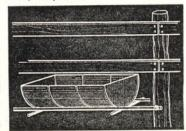
A barrel cut lengthwise makes a solid, economical fence-line feeder. After thoroughly washing the barrel, weld it to steel pipe and bolt the pipe to the fence posts.—C. C., Wisconsin.
