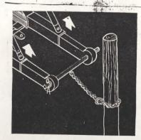
To pull posts easily with a 3-point hitch, we added this 2-ft. piece of %-in. steel bar. We welded a chain and hook to the middle of the bar and drilled holes for clip pins near the ends.—H. S., Kansas.
