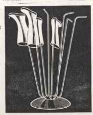
Keep stored boots dry with this boot rack made by welding re-rod to a disk blade. Bend the tops just enough so boots slip on easily.—D. B., Indiana.
