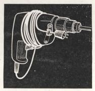
Bolting a spring metal clip to your drill allows you to keep cord wrapped tightly around drill for storage.—
