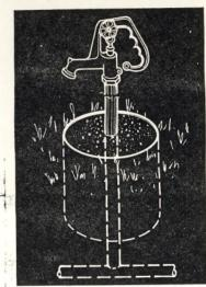
By placing a 12-in. section of pipe filled with sand in the ground around a water hydrant, we reduce the possibility of breaking the hydrant in accidental collisions.—W. S., Kansas.
