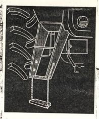
This additional step makes it easier to climb into our tractor cab. It's best to hang the step with two pieces of roller chain so it swings in and out but not back and forth thus avoiding the tire—E. C., Indiana.
