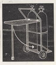
This hinged table flips up for handy welding and stores folded up against the cart.—B. C., Illinois.
