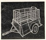
We built this two-wheeled stock trailer from the old box of a pickup truck. Just cut the frame off and weld a hitch to the front of the box. It's a handy way to move livestock from farm to farm.—
