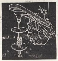
Our three-point mounted post-hole digger can also be used to roll up fence. The regular auger is replaced with a length of pipe with two disks welded in the center. A small pipe driven in the ground slips into the fence roller and keeps it running straight.—C. S., South Dakota
