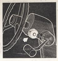
To read hydrostatic control numbers at night, we use a red clearance light mounted on the combine steering column. To prevent distracting glare, the light is painted black inside and out except where it shines on the control lever numbers.—D. E., Illinois.
