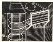
This safety platform built below the roof vent of our grain bin makes it easier to work on stirration equipment and is a handy platform to take grain samples from. We also used small tubing to make a safety cage around the ladder on the bin. The top two rungs extend to the platform so the area is entirely enclosed. D. P. Journ
