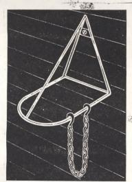
Keep chains hanging neatly with this frame made from ¼-in. or %-in. steel rod lag-bolted to the wall.—R. M., Indiana.
