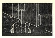
To keep the big doors on our building from blowing open we cemented a pipe in the ground just below ground level so we can drive over it. When the door is closed we drop a smaller pipe into the large one to block the door shut.— C. K., Maryland.
