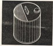
We cut half the top out of a rinsed 5-gal. chemical can to make a handy container for draining oil out of our tractors. This doesn't weaken the handle and lets us easily carry and pour the used oil.—B. G., Missouri.
