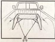
Easily unload sand and gravel from a pickup with this "lazy man's shovel." The <sup>1</sup>4-in. cable is looped through the back and secured with cable clamps. Hook the clevis to a tractor and most of the load can be unloaded without shoveling.—H. K., Missouri.
