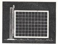
We made this gate with offset hinges so we could vary the ground clearance by turning it upside down. The gate, made of angle iron and 16-in. rod, uses a removable rod as a hinge pin. —D. A., Iowa.
