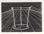
We built our own grain spreader with an old disk blade. Weld three pieces of rod to the disk and bend a hook on one end of each to hang it from the lip of the bin. We hang ours about three feet below the top of the bin.—D. S., Minnesota.
