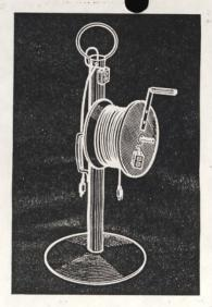
Make this portable power pole by welding 1½-in.-diameter pipe to an old disk blade. Axle for cord reel is a piece of ½-in. pipe welded to the stand.—L. S., Iowa.
