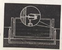
To cross a gate opening with our electric fence wire, we buried a length of 1-in. galvanized pipe under the driveway and ran insulated wire through the pipe.—B. I., Iowa.
