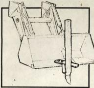
We made a wood-post puller by welding two old rotary-mower blades together. One person holds the post against the blades while the loader is raised.—
