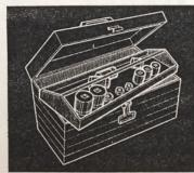
Sockets stay orderly and easy to find since I fastened a nut for each size socket to the toolbox. The sockets slip onto the nuts and stay in place. — H. A., North Dakota.
