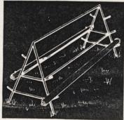
We made this handy iron rack in the shape of an A-frame.—C. W., Iowa.
