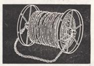
Barbed wire is easy to unroll using this pull cart we built. The two wheels make the cart easy for one man to pull. —D. G., Nebraska.
