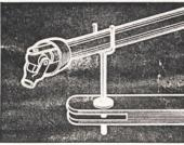
This stand drops in the hitch pin hole to keep the PTO shaft off the ground when an implement is unhooked. Clip it on the implement when not in use.—
