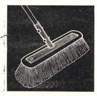
Our shop broom handles don't break anymore since we reinforce them with a piece of sheet metal and length of pipe. Insert the wooden handle through a hole in the sheet metal and then weld the pipe on the handle to the sheet metal.—D. B., Indiana.
