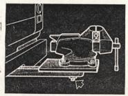
Our portable vice is carried in the toolbox of our pickup until needed. Then it is attached to the hitch with a large bolt welded to the bottom of the mounting plate.—T. H., Ohio.
