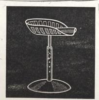
This handy shop stool was made from parts out of our scrap pile. A disk blade is used for the base and an old tractor seat for the seat. The seat height is adjustable as two pipes slip inside each other and can be pinned in place.—J. Z., Indiana
