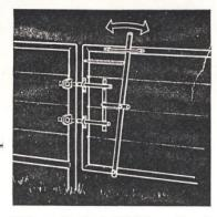
This spring-loaded latch makes it easy to open and close our swinging gate. The handle and latch bars must both pivot for smooth operation.—
