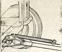
An old plow spring helps make heavy wagon tongues easier to lift. — L. L., lowa.
