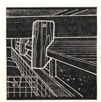
Free both hands for lifting modified open-front hog-house panels with these latches made from ¾-in. plywood or 2x6-in. lumber. When raising panel, it hits lower incline, latch swings open, then locks into place. When closing panel, a quick push against upper incline swings latch open; door can then drop past latch. A large, removable nail in drilled hole holds latch in place when panel is up.—E. S., Nebraska.
