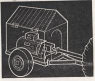
A trailer built under our standby generator makes it portable and a "dog house" protects it from the weather. There is also room on the trailer for our welder.—G. A., New York.
