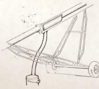
We collect screenings from our auger with the help of a section of U-trough clamped below the screening section. The screenings are caught in the U-trough and funneled to buckets or a wagon through a piece of plastic drainage tile. — R. D., lowa.
