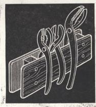
Handy wall holder for pliers and Vise-Grips is made by nailing ply-wood to blocks and mounting on the shop wall.—A. H., Pennsylvania.
