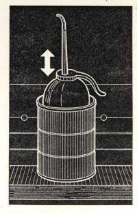
A tin can bolted to the floor or fender of our equipment makes a good place, to store oil cans. Can won't roll around and spill and is always handy when needed.—B. W., South Dakota.
