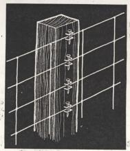
For easy-to-remove temporary wire fencing or stock panels, I drive large staples above and below the wire. A nail slipped through each pair of staples holds wire.—T. L., California.
