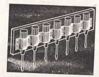
This screwdriver holder is made from a narrow strip of inner tube and is mounted along the wall of our farm shop.—J. M., Nebraska.
