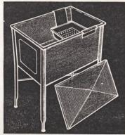
We made a parts washer from an old rinse tub. The lid and tray are made by bending 24-gauge steel in a sheet metal brake. Tray holes are ¼-in. diameter. —K. C., Nebraska.
