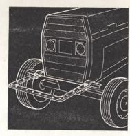
We mounted an old drawbar on the front of our tractor to push and pull wagons around the farmstead. The drawbar is attached to angle iron brackets with two bolts, allowing us to remove the bar quickly and easily. —R. C., Illinois.
