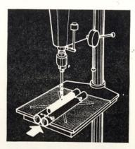
To drill pipe or irregularly shaped objects, I made a V-block out of two pieces of large-diameter pipe bolted together and clamped onto the drill press.—G. R., Illinois.
