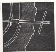
Two large pipes are cemented on the sides of our shop door just inside the door frame to protect it from wide implements. A hump of concrete at the bottom wedges tractor tires safely through the opening.—F. W., South Dakota
