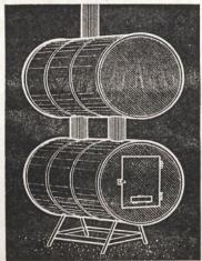
Get your shop ready for winter with this economical wood-burning stove. The stove is built from two used 55-gal. oil drums, stovepipe, an old furnace door and angle iron for the base. The top drum provides additional heating surface.—B.M., North Dakota.
