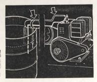
We made an automatic shutoff for the gas-engine powered pump on our livestock watering tank. We ran an insulated wire from the spark plug down a few inches into the tank. A second wire runs from the tank to a ground on the engine shroud. When water rises to the level of the two wires, the engine grounds out, shutting off the water.—
