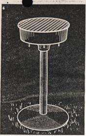
We made this sturdy grill by welding an old brake drum on one end of a pipe and a disk blade base on the other.—
