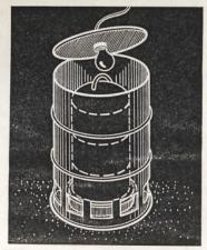
This inexpensive heater keeps our chicken waterers thawed out in the coldest weather. It's built from a 30-gal. barrel and a heat bulb.—H. H., Illinois.
