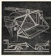
We improved the towing traction of our 2-WD pickup with this frame of welded tubular steel. It raises the tow line, putting more force down into the wheels.—S. C., Florida.
