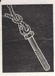
To ease unhitching, we wild hex nuts to hardened bolts which serve as hitch pins. A tug on a rope tied through the nut lets us unhitch from the tractor seat.—B. L., Nebraska.
