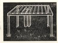
This boot rack helps keep overshoes clean and dry. We made it out of narrow angle iron and keep it just outside the barn.—B. H., Iowa.
