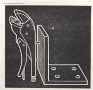
This handy portable vise bolts to any of several workbenches in my shop. I made it by welding a pair of Vise-Grip pliers to a bent piece of ¼-in. flat iron.
