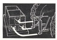
We made our hog feeders portable by equipping them with stirrups that enable us to use the three-point hitch on our tractor. The three heavy iron bars are welded to large pieces of flat iron which are bolted to the side of the feeder. This is especially handy when we're scraping lots or moving feeders from pen to pen.—L. B., Iowa
