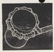
We made this tool to remove oil filters by attaching a piece of #50 roller chain to a %-in. rod which has been ground flat on one end. Holes in the rod to hold chain are 1¼ in. apart.— C. B., Wisconsin.
