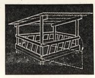
We built this wooden round bale feeder to keep hay dry. It is 7 ft. square with the floor 2 ft. off the ground and the roof 8 ft. high. One end swings open to fill the feeder.—C. M., Missouri.
