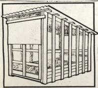
Keep round bales dry with this homemade feeder. Made of rough-cut oak and plywood, the feeder opens on one end to hold two 5'x6' bales. - G. H., Arkansas.
