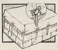
To securely hold plastic covers on hav, we place a smooth pebble or glass marble under the plastic, then tie twine around it. The twine will not slip or tear the plastic. - H. C., Pennsylvania.
