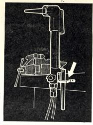
We mount a small light on the end of our combine unloading auger and shine it where the grain will fall in the wagon. This lets us know when wagons are full at night.—T. D., Iowa
