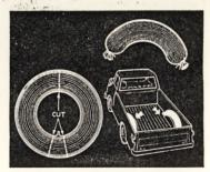
Improve pickup traction by cutting innertubes, filling them with sand and tying the ends. Mounted over the wheel wells, these weights leave the bed free and provide sand which can be spread on ice for traction when stuck.—M. C., Colorado.
