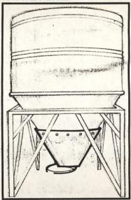
I made this bulk bin for ground feed by rebuilding an old hog feeder. Remove the trough, take the cone out of the inside and bolt it to the outside. Then add a door to the bottom. - T. K., lowa.
