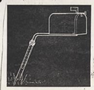
Our mailbox swivels when bumped by passing snowplows, then is pulled back into position by gravity.—C. L., New York.
