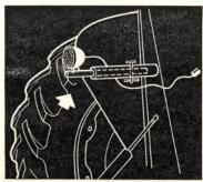
We built a removable light for our tractor by mounting a headlamp on a small piece of pipe that slips into a larger pipe that is bolted to the tractor fender. Extra electrical wiring running to the light makes it portable for nighttime repairs on the tractor or equipment.—G. T., New Jersey.
