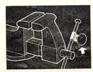
We've always had problems running our vise in and out, especially when it was mounted so the handle ran close to the edge of the bench. To solve the problem we clamped a steering wheel spinner on the handle. Now we can run the vise in with one hand and not nick our fingers.—R. L., Nebraska.
